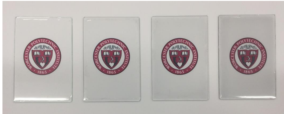
Figure 15- Optical view of 80 \mu m thin films of MoS 2 /PDMS composites on glass slides (from pristine PDMS on left, to 0.1wt.% MoS 2 /PDMS on right).
