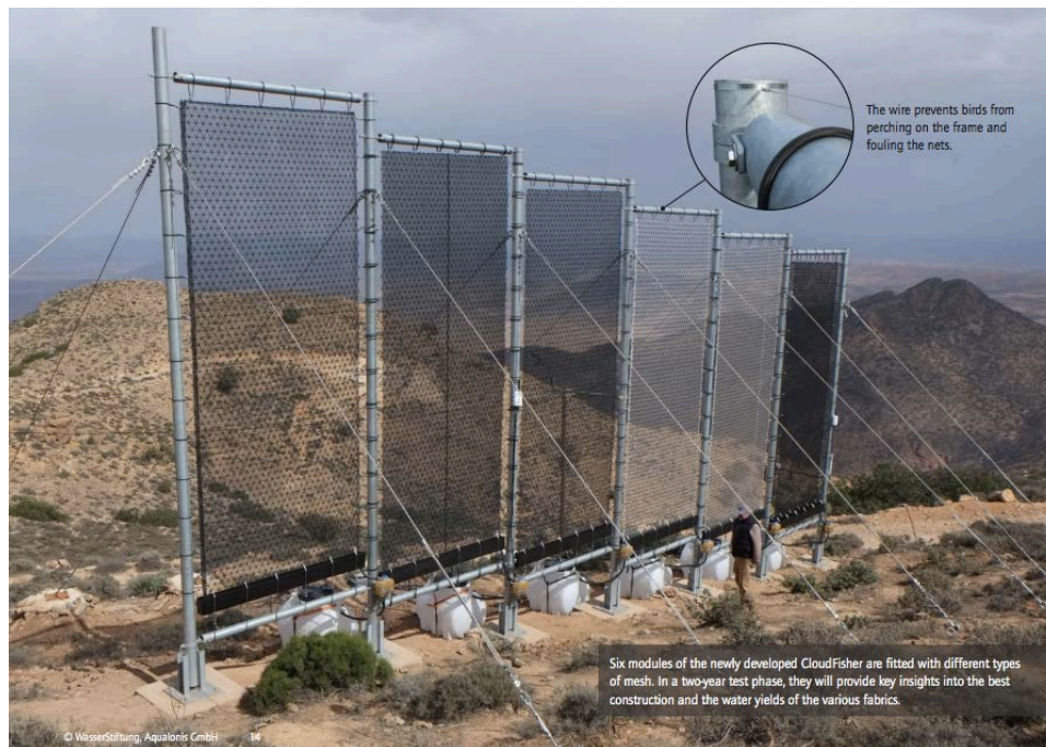
Figure 21: Six modules of the next-generation nets with different types of mesh (Aqualonis, 2015)
