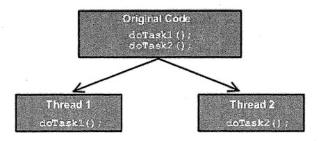
Fig. 4.5: Functional (Task) Decomposition
