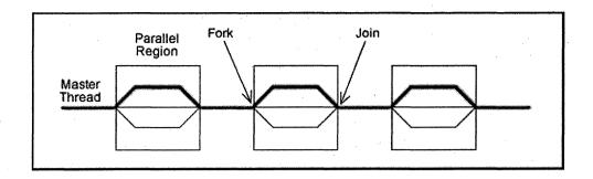
Fig. 4.7: OpenMP Parallel Region/Fork-Join Model
