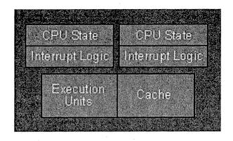
Fig. 2.2: Simultaneous Multi-Threading Architecture
