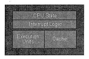
Fig. 3.1: Single-Core Architecture
