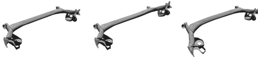
Figure 2. Modal space reduced finite element (FE) model: Screen-shots from an interactive simulation of a car rear-axle.
