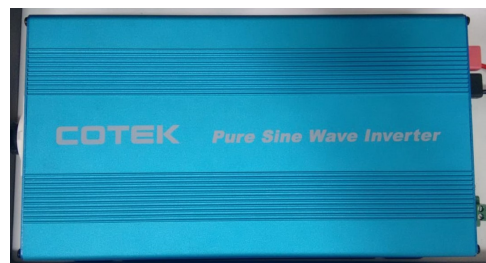
Figure 5.14: Inverter Cotek 600 W.
