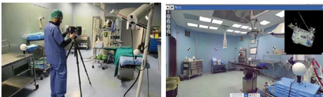
Fig. 1 - Survey with a terrestrial laser scanner in an operating theater and point cloud processing, within Autodesk RECAP software.
