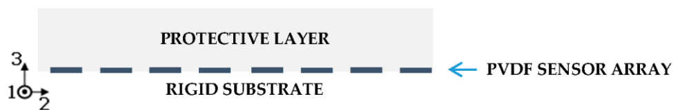
Figure 1. The PVDF sensor array is located on the bottom of the protective layer and integrated on a rigid substrate (side view).
