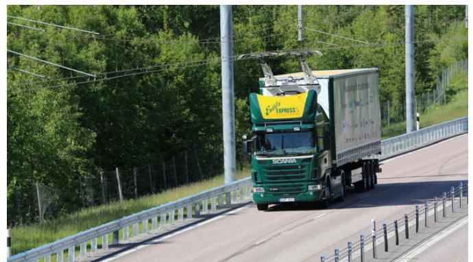
Fig. 5. Scania's truck being powered via overhead electricity lines [42].
