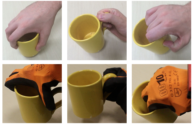
Fig. 2. A human hand grasping a cup with three different approaches (top panels) and the same grasps reproduced with the Pisa/IIT SoftHand (bottom panels).
