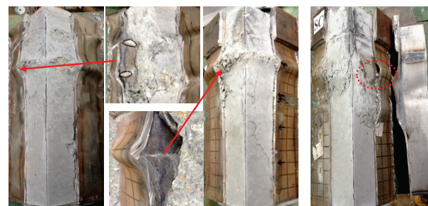
Figure 10 Observed interior damage
