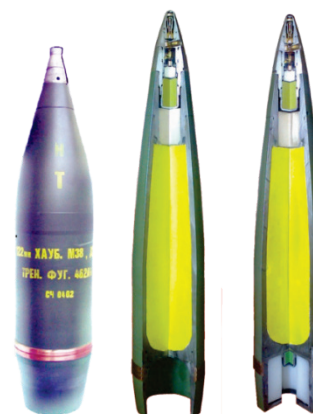
Figure 2. The projectiles used in this study (from left to right): standard projectile (122_ST), the hollow base projectile (122_HB) and projectile with base bleed (122_BB)
