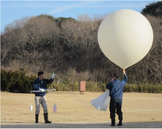
Figure S1: Preparations for a flight launch at 8:30 local time on January 6, 2017. RS-11G and RS92 radiosondes were hung at the two ends of a plastic cardboard rod.
