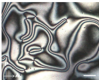
Figure 2. Polarized optical microscopic image of pyrene-based cyclophane 1 at r.t. in the absence of a coverslip. Scale bar: 20 μm.
