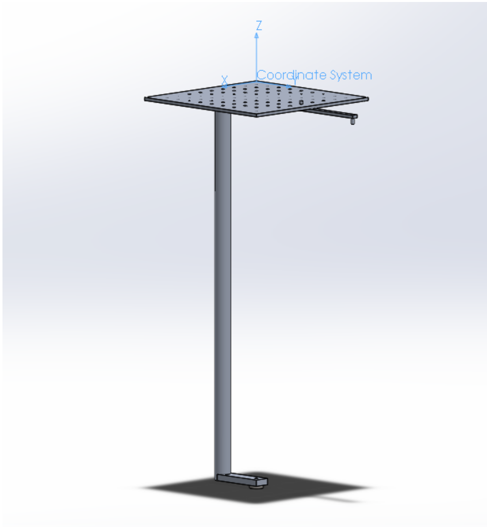
Figure 5.1: Oscillatory components of the pendulum and frame of reference used for the calculations of the centre of mass and the Z-component of the inertia tensor I_{ZZ} of the system. Components shown in the Figure are the oscillatory support column, the oscillatory arm with laser, the oscillatory satellite platform, and the lower and upper bearings (inner or mobile cylinder).
