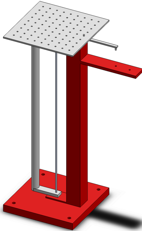
Figure 3.12: Complete pendulum assembly; Grey-colored: Oscillatory components of the torsion pendulum; Red-colored: Fixed components of the torsion pendulum
