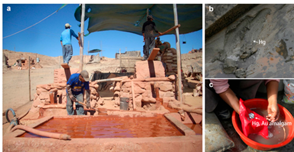
Figure 4. Gold recovery by artisanal miners in the Nazca-Ocoña area. (a), grinding with the mill quimbalete; (b) Hg-rich concentrate; (c) miner obtaining the amalgam.
