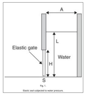
Rubber is a nonlinear material, however in the present study linear elastic approximation is used. The value of the Youngs modulus is approximated here as  $0.5(E_0 + E_{100})$ , where  $E_0$  is the Youngs modulus of the virgin material and  $E_{100}$  is the value that corresponds to the deformation of 100% (these values are taken from [9]).
