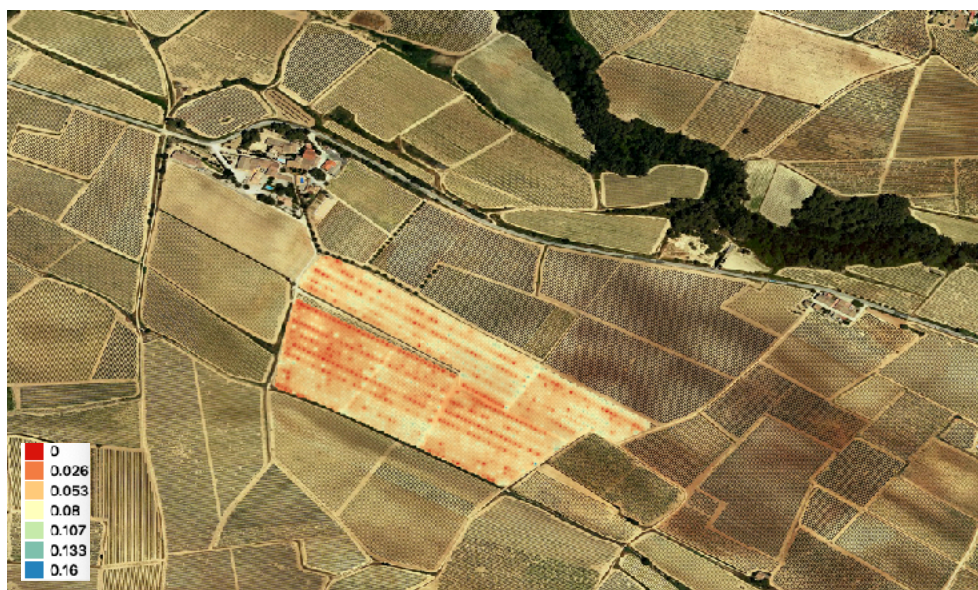
FIG 29: 9th May. Geolocated field moisture map over orthophoto. Volumetric moisture optimised to retrieved value range - 0 to 16%
