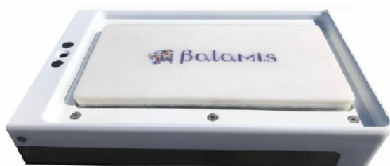
Balamis dual antenna mobile L-Band radiometer with photodiode mounts (left)
