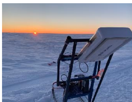
FIG 5: Climate change models often have a large predictive error range due to lack of detailed local process data eg. 90 year temperature change forecast of Arctic sea ice (left) and a mobile, sled mounted radiometer for ice thickness (photo: Lars Kaleschke).
