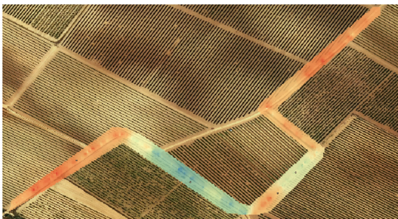
FIG 20a: Emissivity (06 May) A seven level equal interval classification using inverse distance to power in QGIS. Note that samples were taken in a single row and the interpolated width is exaggerated.
