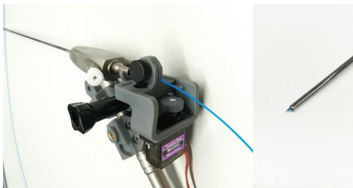
Figure 12. The laser tool to produce the coagulation of the anastomosis points and the extraction/retraction actuator
