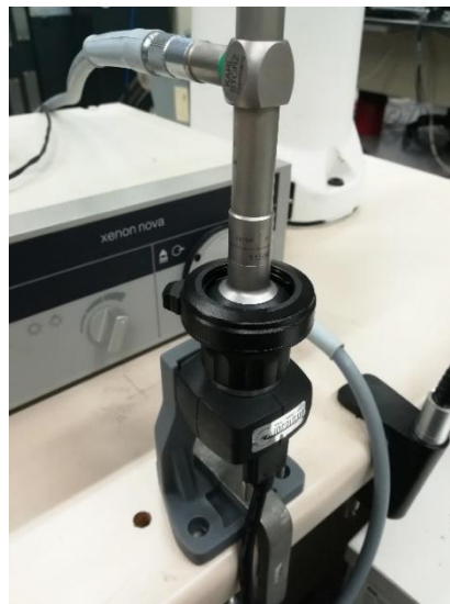
Figure 11. The fetoscope camera that sends the images to the user interface
