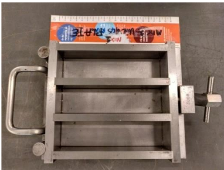
(a) Prism mold used in the casting.
