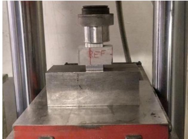
(b) Set-up in pressure machine Tony 300.
