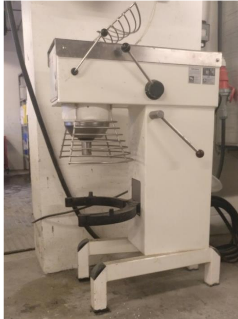
Figure 9.4. Hobart Mixer for high volume mixtures used for the experimentation.
