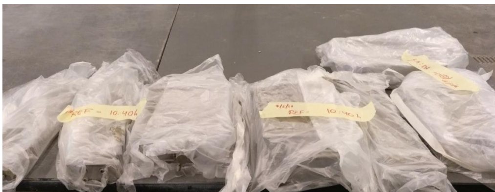
Figure 9.6. Specimens after casting covered with plastic during 24 h.
