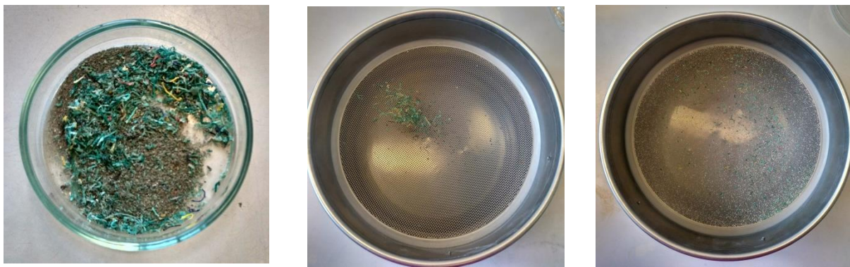
(a) Sample of 60 gr of 'green' PE fibers and impurities.
