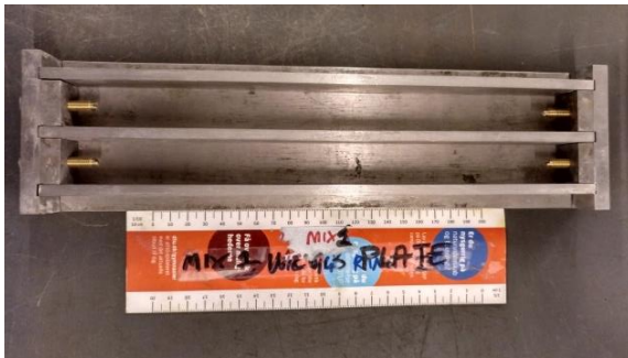
(a) Bar mold used in the casting.
