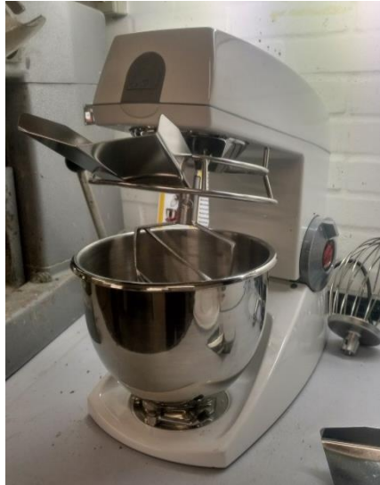
Figure 9.7. Hobart Mixer for low volume mixtures used for the experimentation.
