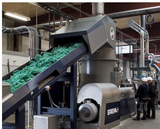
Figure 13.2. Processing and cutting of discarded fishing nets in Plastix installation.
