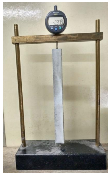
(b) Micrometer with bar specimen.
