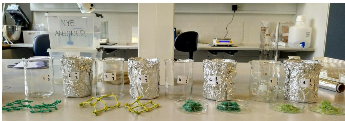
Figure 5.2. Preparation of the set-up for the microplastic release experimentation.
