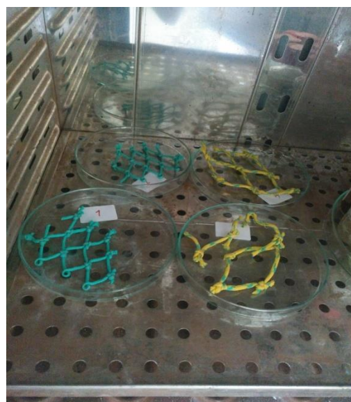
Figure 5.6. PE small scale fishing nets drying into the oven.
