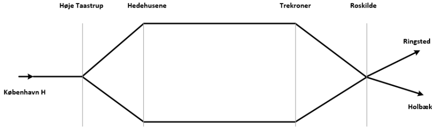
Figure 5.9: Illustration of the quadruple-track segment for the trains in direction out of KH
