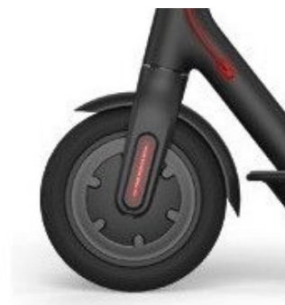
Figure 2.21 Electronic brake in the front wheel. (From Xiaomi M365)
