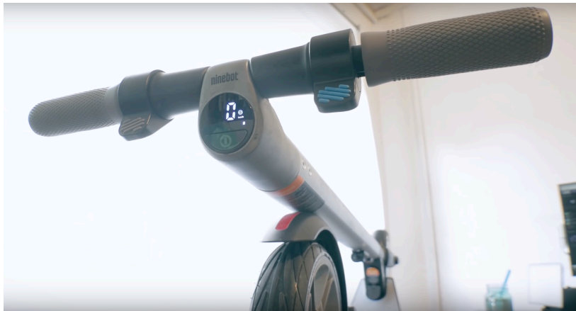
Figure 2.22 Ninebot ES2 handlebar (Right lever: Accelerator, Left lever: Brakes)
