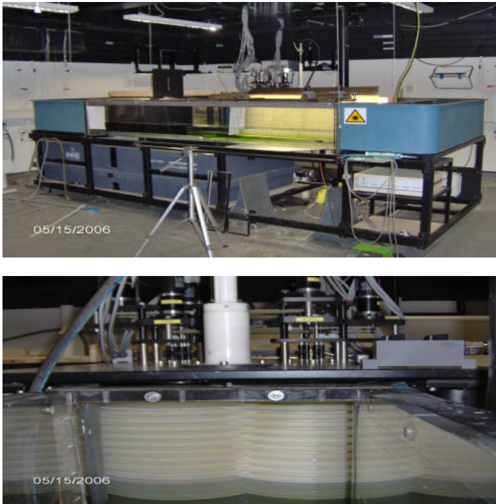
Fig. 8. Racetrack type of shear-stratified tank designed by [16] used for the LIF visualizations and the conductivity measurements on grid collapse (above) general view, (below) details of the disk pump.
