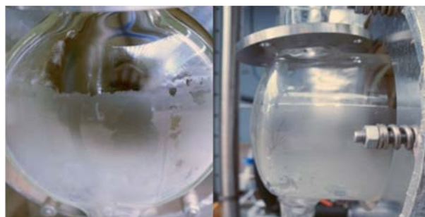
Fig. 11. Scale formation on Re-boiler wall.
