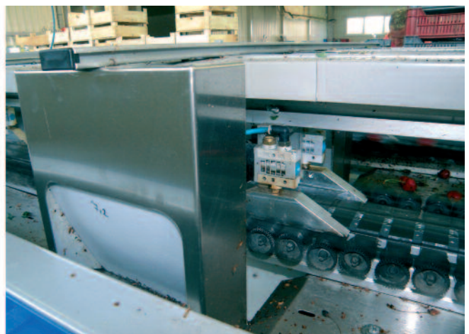
Fig. 8: The air separation units
