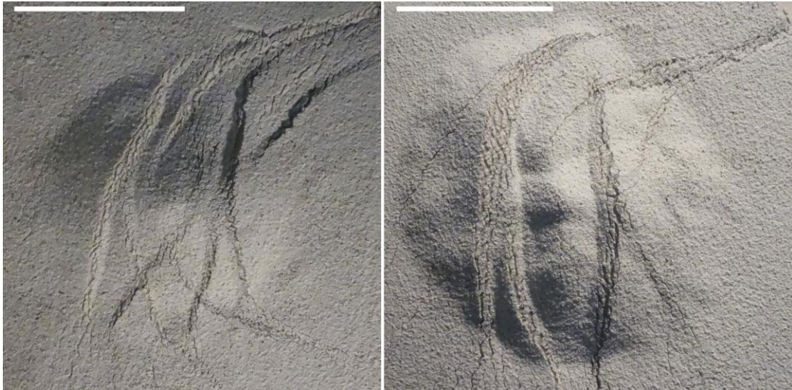
Fig. 6. Two analogue models of sand and plaster cones on a sand apron overlying a silicon putty basement sloping 2^\circ towards the right, representing Mt Etna's brittle summit cone and apron of lavas overlying the sloping ductile basement beneath it. Left and right images were taken 43 and 40 minutes respectively after the start of the experiments. Illumination is from the lower right in the left model, and from the upper right in the model on the right. Key parameters in both models are scaled to match those at Mt Etna. The left model was a simple flared cone, whereas the right model was elongated north-south in an attempt to represent the Northeast rift and the Piano del Lago. The cone heights were 45 mm, the sand apron thinning from 20 mm beneath the cone to 8 mm to the right. The silicon thickness was 12 mm in the left model and 14 mm in the right model. Both models have a prominent summit graben complex that runs into a left-lateral strike-slip fault system similar to the Pernicana Fault on Etna (fig. 1). Scale bar is 10 cm.
