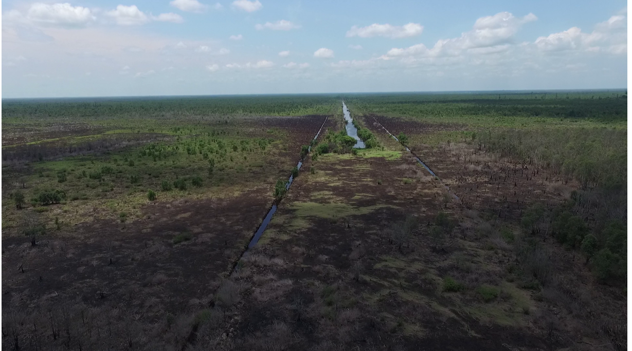
Figure 2.6: A view of the Kalampangan Canal looking north-east from the Sabangau River (out of shot). The canal drains two peat domes along its 12 km length, reaching the Kahayan River in the southeast. The canal does not directly discharge into either river but at its ends which terminate ~200 m from the river, there are parallel 'feeder' canals which receive the main canal's waters and channel them into the rivers. It was these feeder canals that were sampled in the investigation.
