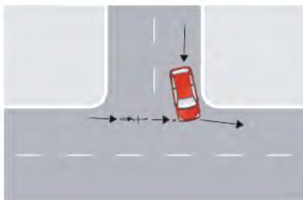
Figure 4.8 Example of an ‘Intersection: thru-left’ crash at a priority control intersection: RUM 17 (n=2 group rider and 3 individual rider crashes)
