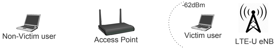
Fig. 1: Scenario shows a Wi-Fi AP with two users and an LTE-U eNB both operating on the same unlicensed channel. The victim Wi-Fi user is inside the influence zone of LTE-U; and the non-victim Wi-Fi user along with Wi-Fi AP are outside the influence zone of LTE-U.
