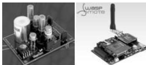
Fig. 2.8: Libelium Wasp mote and various gas sensor panel
