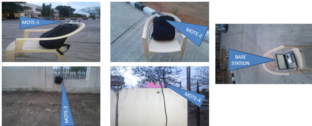
Fig. 2.10: IITH's wireless air pollution monitoring system
