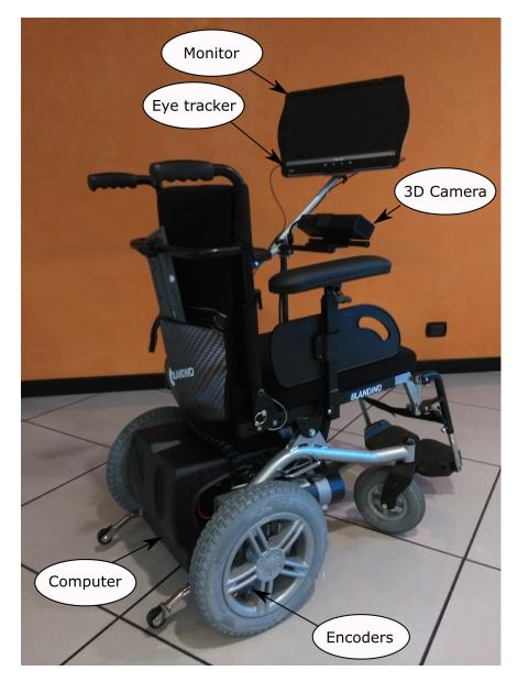
Fig. 5.6 Prototype of semi-robotic eye controlled wheelchair.
