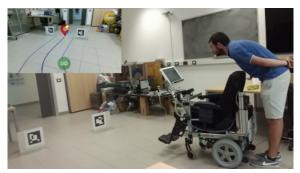
(a) The activation of the manoeuvre by gazing the pin for 2 seconds
