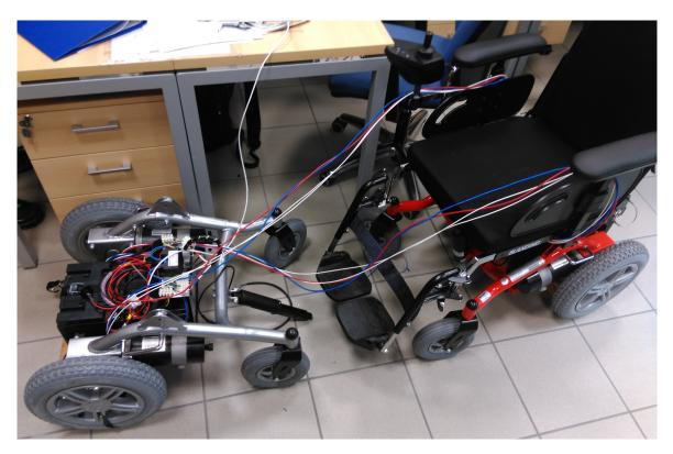
Fig. 5.12 Testbed for the calibration of the wheelchair kinematic parameters.
