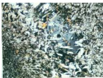
Fig. 3. Stripe of coarse-grained rhodonite in fine-grained rhodonite mass. Magnification 50x, N+
