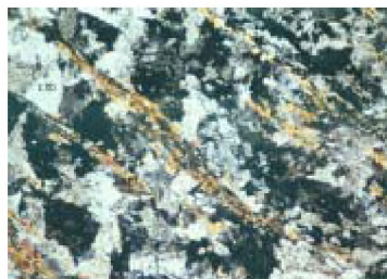
Fig.2. Microphotograph of grey blue grains of rhodonite with epidote stripes, magn. 50x N+
