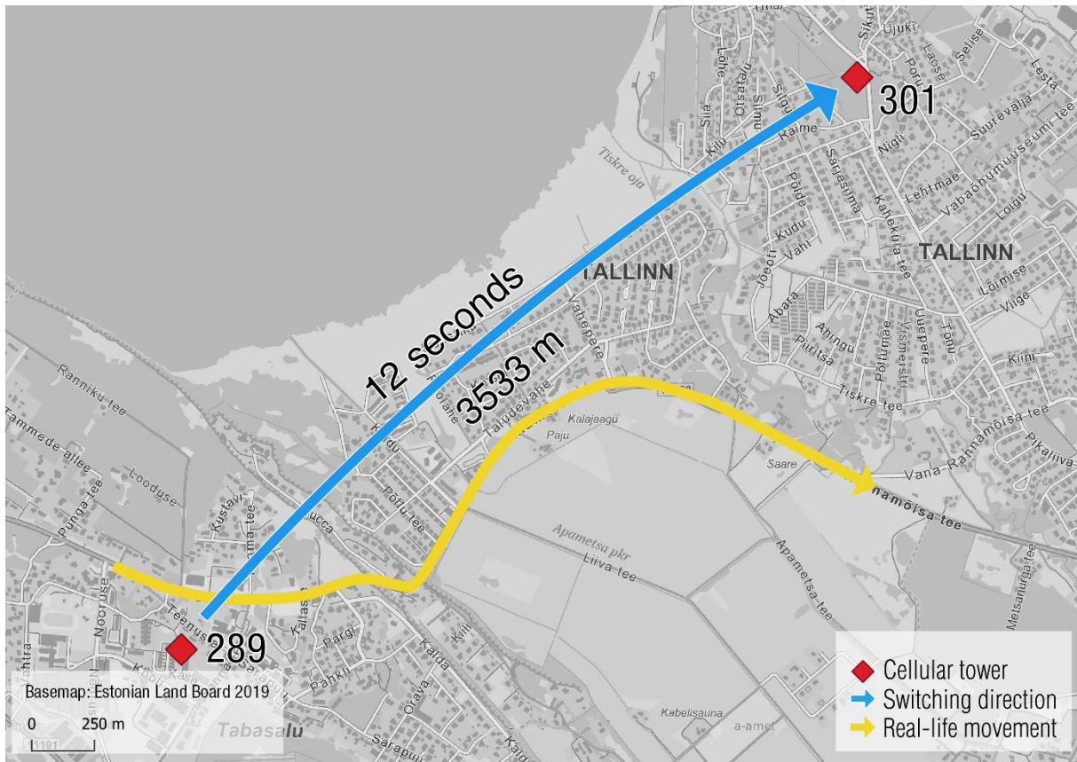
Figure 10. A stable period in the coverage area of cellular tower 289 is followed up with a log in 12 seconds from cellular tower 301, which is 3533 meters away. The user travelled by car in the shown direction.
