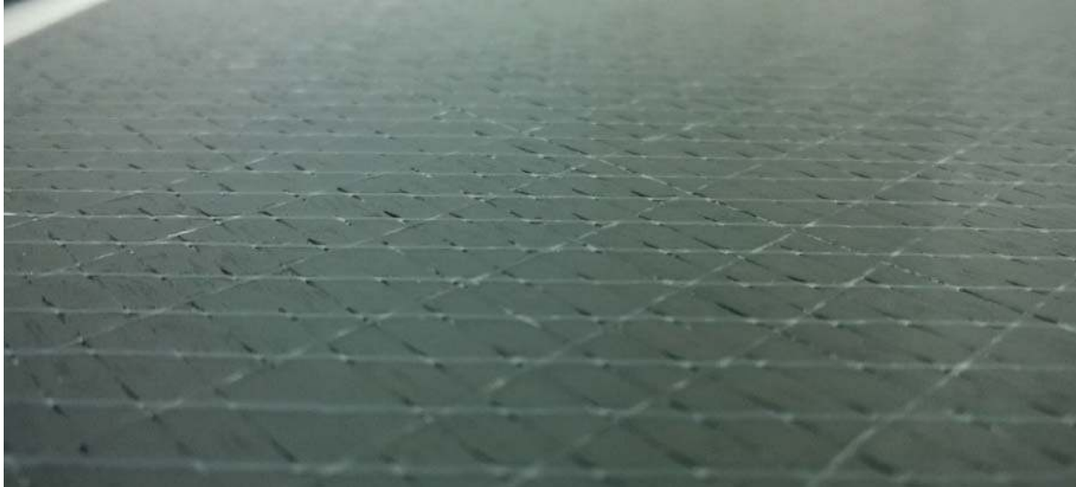
Fig. 3. Example of a CFRP specimen with porosity
