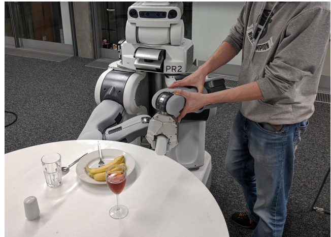
Figure 1: Example setup - task is to return the pepper shaker to its original location—next to the salt shaker. Deciding which objects to avoid when performing the task can be seen as conditioning on the user specifications, implicitly given during a demonstration phase.
