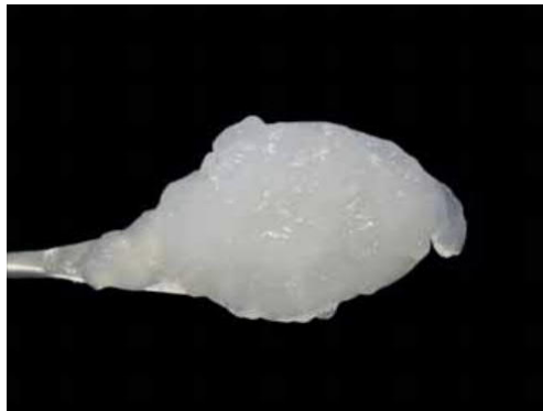
Figure 17. Mechanically extracted (enzymatically pretreated) 2 wt% CNF suspension obtained from eucalyptus (Lavoine et al. , 2012).
