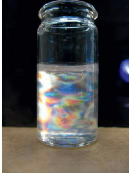
Figure 19. Capim dourado cellulose nanocrystals between cross-nicols showing the birefringent domains (left) and Transmission electron micrograph image of ramie nano crystals (Siqueira and Abdillahi, 2010).
