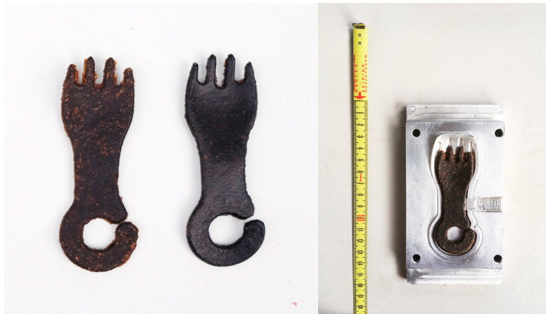
▼ Extruded samples. Right: material shrinkage after drying.
