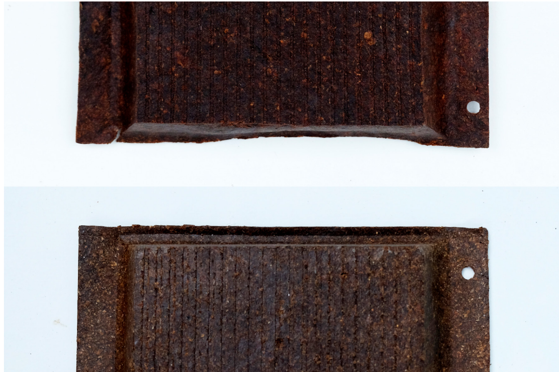
▲ The lower sample has extended edges, which made the walls more stable and less deformed.
