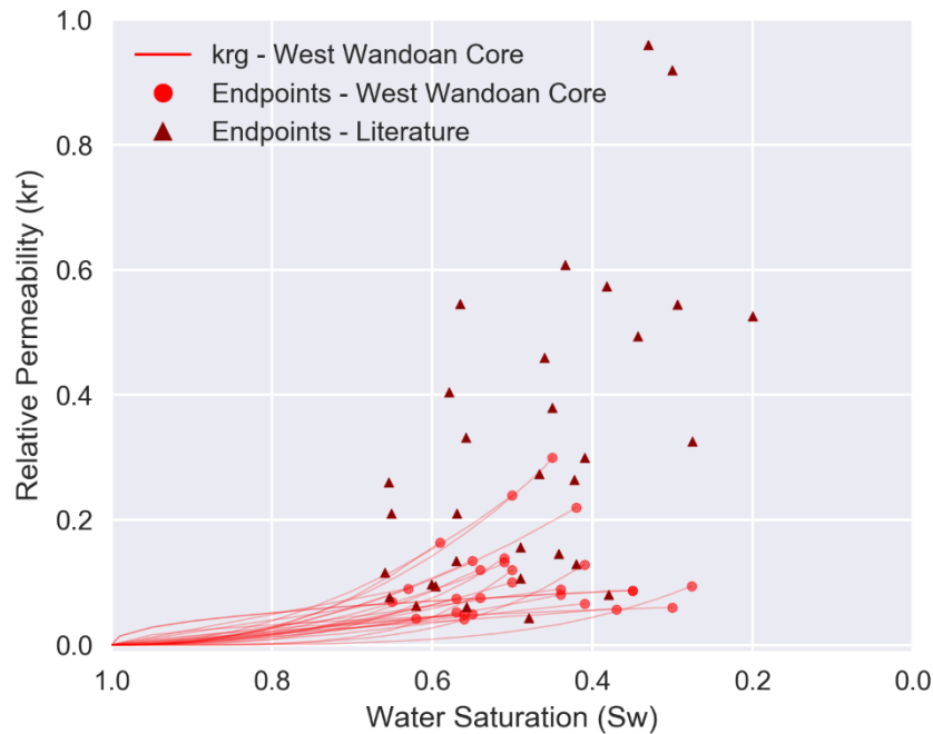
Figure 2 Drainage CO 2 relative permeability endpoint data from literature (triangles) and the West Wandoan 1 well core analysis (circles).
