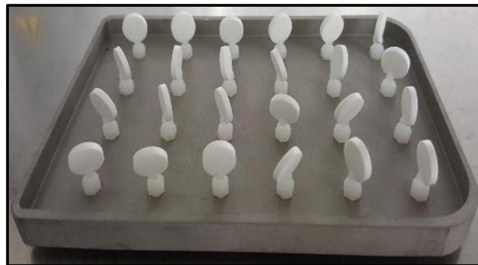
Figure 7. AAA biofilm model with the mounted HA discs
