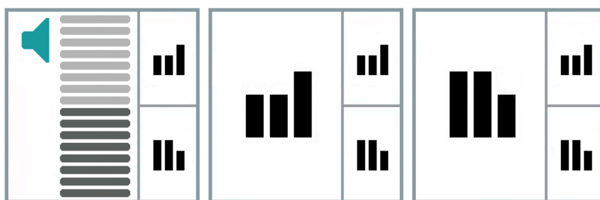
Figure 6-2. Representation of the remote control display when changing the volume (left), increasing the sharpness (middle) and decreasing the sharpness (right).
