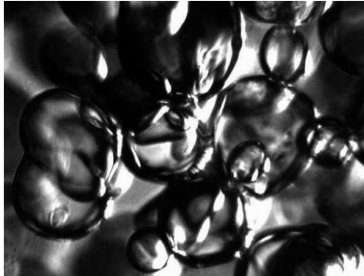
Figure 3.1. Microscopic photograph of a sample ice slurry [44].
