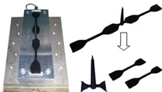
Fig. 7 Production of test samples by injection molding
