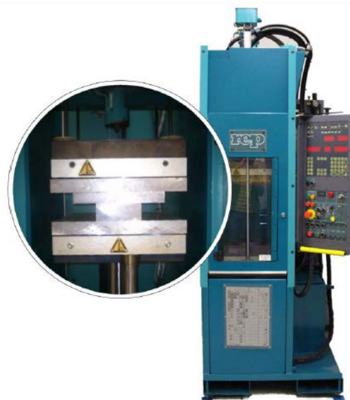
Fig. 6. Injection molding machine REP V27/Y125
