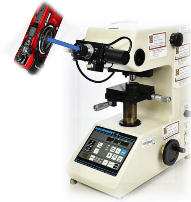
Figure 5.12 – Taking the microscopic photographs through the microscope of the Knoop micro-hardness tester using a camera.
