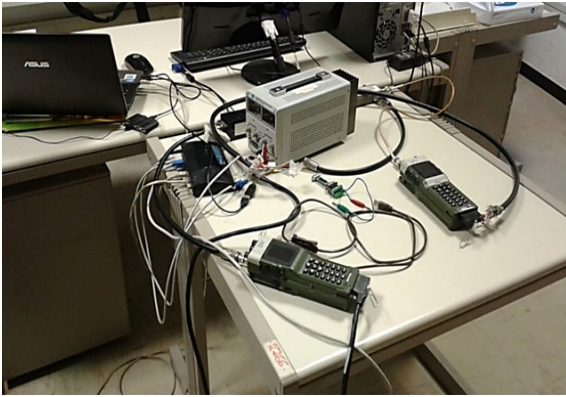
Fig. 2: SDR testbed utilised to generate the dataset with wideband spectrum measurements: hardware platform.
