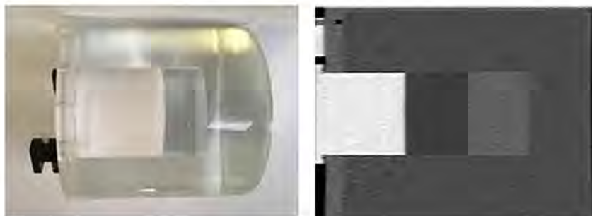
FIG. 1. Photo and sagittal view of the TTF phantom filled with water with its different contrast rods: PTFE, polyethylene, and PMMA.
