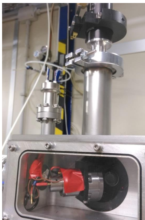
Figure 39 Experimental setup at Elettra: the cell is placed inside a vacuum chamber connected to pumps
