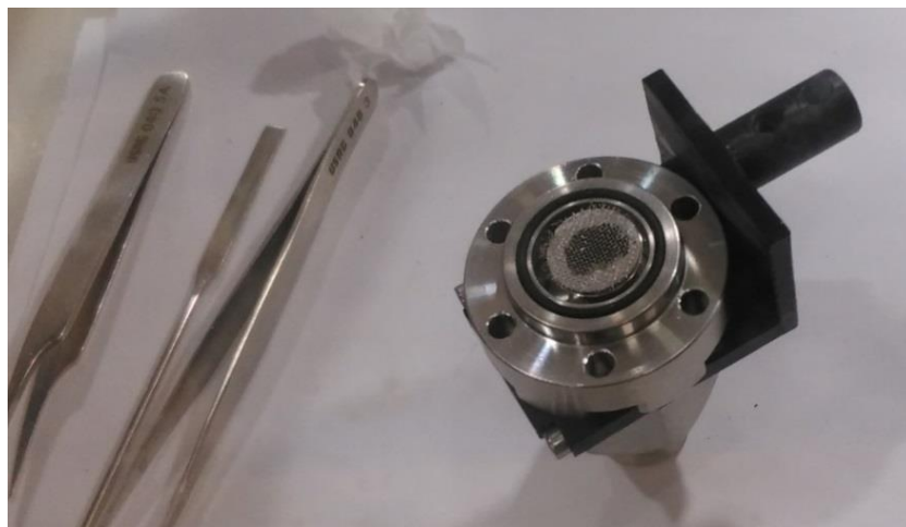
Figure 38. Cell for in-situ measurements for Elettra showing steel current collector and cathode material
