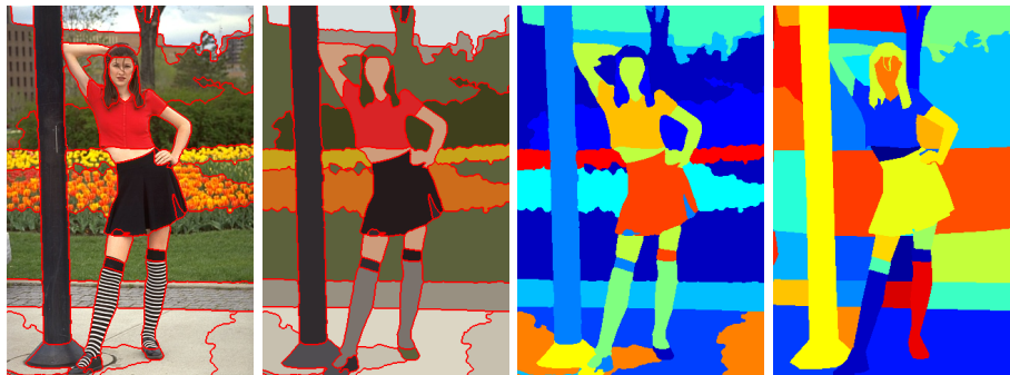
Fig. 2. Example demonstrating the global property of the spectral segmentation when employing our full-range affinity. All instances of grass, sky, skin and orange tulips belong to the same regions. Left: the original image with segments found using our method outlined in red. Middle left: average colors within segments. Middle right: segments in false colors. Right: manual segmentation from BSD3 shown with false colors [1] lacks the global property.
