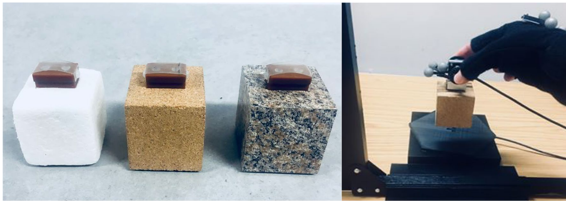
Fig. 1 The expanded polystyrene, corkwood, and granite objects lifted by participants (a) and the experimental set-up during a lifting trial (b)
