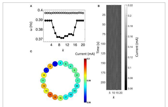
**FIGURE 2** | Experimental traditional chimera state in a non-locally coupled regular network. **(A)** Frequency of the oscillators. Open circles: natural frequency. Solid circles: frequency with coupling. **(B)** Space-time plot of the current in gray scale. **(C)** Snapshot of the current of the electrodes.  $V = 1,094 \,\text{mV}$ ,  $R_{\text{ind}} = 1 \,\text{kOhm}$ ,  $R = 499 \,\text{kOhm}$ ,  $C = 4.7 \,\mu\text{F}$ .
