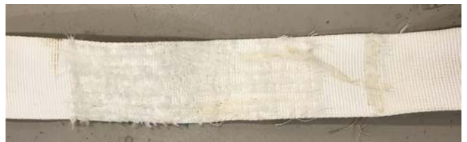
Fig. 10. Sample 3-SKB. Complete belt loop failure at MBS = 144.9 kN.
