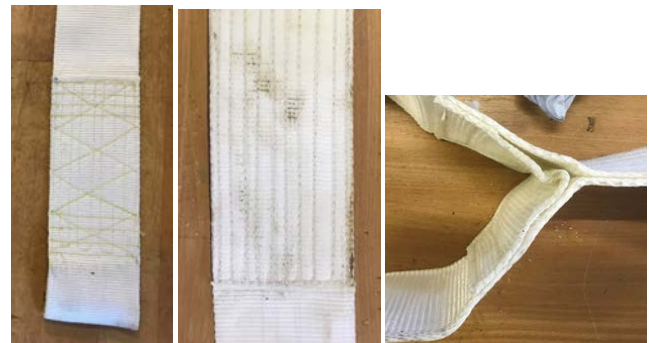
Fig. 2. HDPE mooring belts – loop stitching. Left – Sample 1-TTS closeup of loop stitching. Centre: Sample 3-SKB closeup of loop re-stitching. Right: 3-SKB closeup of reinforcement strip in belt loop.
