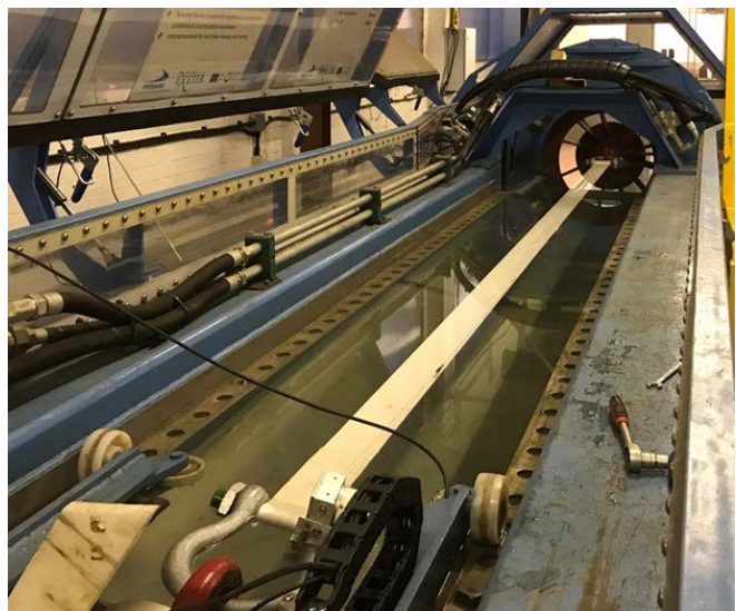
Fig. 1. Experimental setup in the Dynamic Marine Component test rig. Top figure: Engineering Drawing and conventions. Bottom figure: Installed and submerged test sample connection to the hydraulic actuator.
