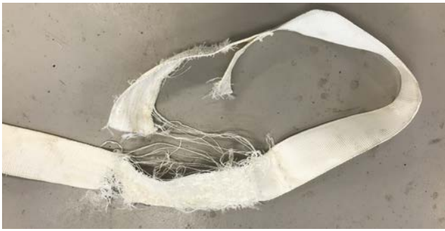
Fig. 11. Sample 4-SKB. Complete belt loop failure at MBS = 205.9 kN. Two failure mechanisms were observed; failure of the stitch and a transverse tear across the belt.
