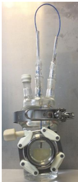
Figure 36: Custom made reactor vessel attached with fused silica viewport, with a single looped wire connecting the working electrode to the Pt mesh counter electrode. Used in hydrogen evolution test.
